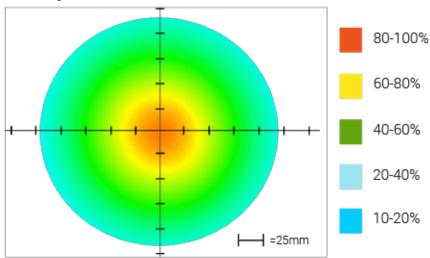
Optical measurement taken using RL4260-625100Li3 @ 300 mm
