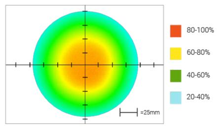
Optical measurement taken using RL113-WHIIC @ 300 mm
