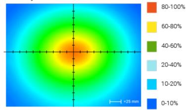
Optical measurement taken using AL295-150WHIIC Rev. A @ 300 mm
